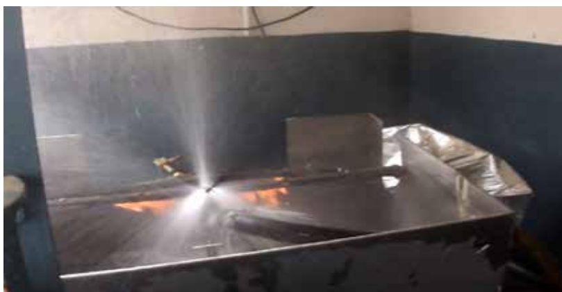
Fig :2 Fixture for Resistance to Fire with Water, Protocol W
