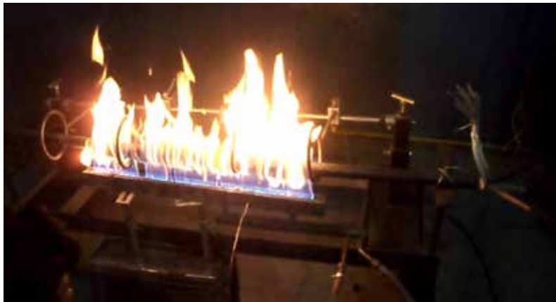
Fig 1: Fixture for Resistance to Fire alone, Protocol C
