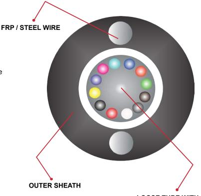
LOOSE TUBE WITH JELLY & FIBRE
