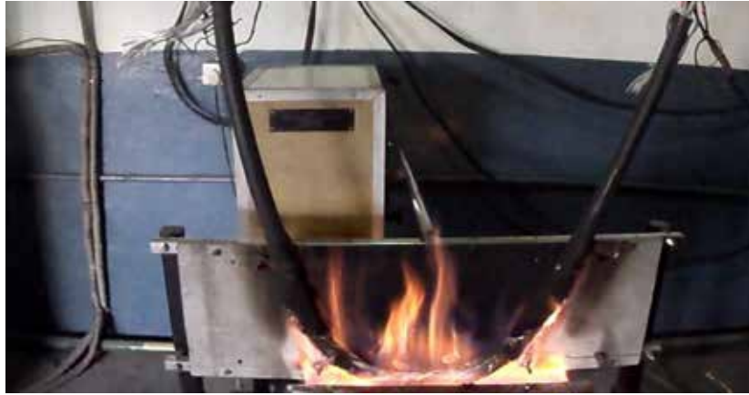
Fig : 3 Fixture for Resistance to Fire with Mechanical Shock, Protocol Z
