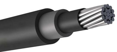
Medium Voltage Covered Conductors consist of a conductor covered with insulating material(s) as protection against accidental contacts with other covered conductors and with grounded parts such as tree branches etc. In comparison with insulated conductors, this covering has reduced thickness, but is sufficient to withstand the phase-to-earth voltage temporarily.
